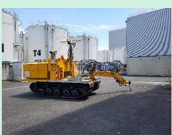
X-ray probe placement by the remotely operated robot ERASE
